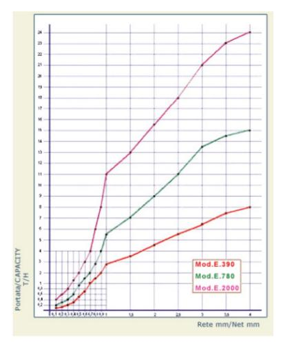
The diagram has been built using wheat flour as the product to be passed through the sieve; its particle size ranges between 0 and 0.2 mm. This diagram is only indicative of the general operation of the separator.
